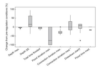
Fig. 3. Interquartile box plots showing percentage change in values from pre- to post-regulation conditions of eight hydrological variables in 24 wetlands. Calculated as: Change = 100 × ((postpre)/pre).
